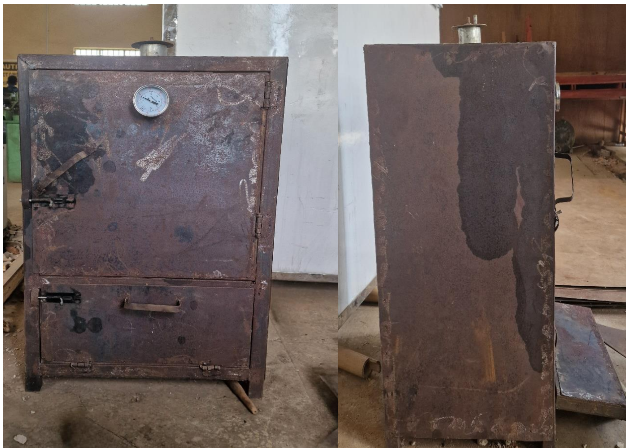
Figure 3. Fabricated dual-energy source baking oven
