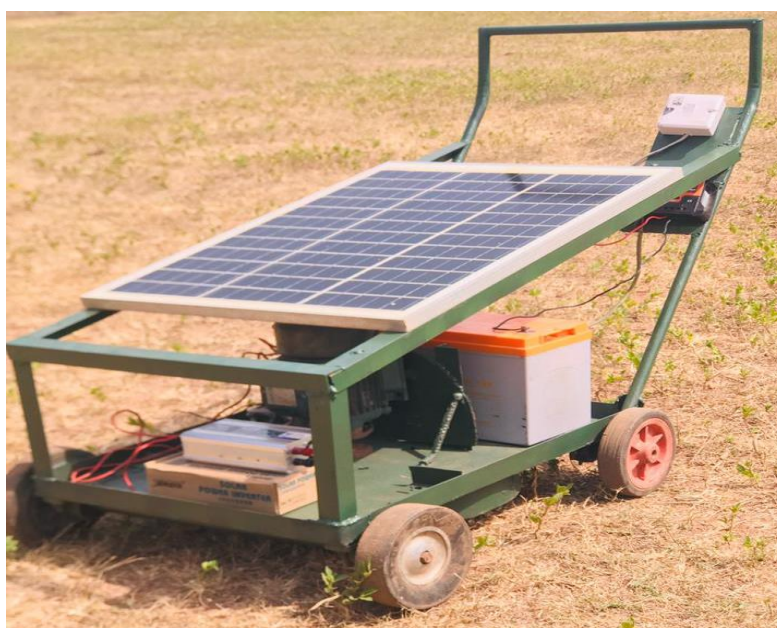
Plate 1: Fabricated solar lawnmower
