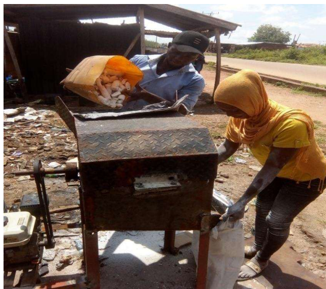
Plate 1: Hammer mill in operation
